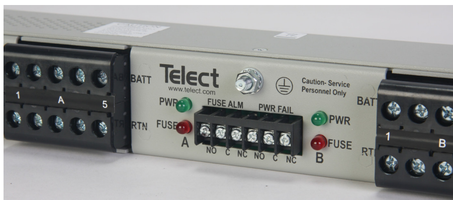
Figure 11 - Status LEDs & Alarm Terminals
