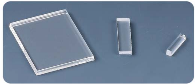
Figure 1: Sample of a PLC-style splitter chip. (Photo courtesy of The Blue Shift.)
