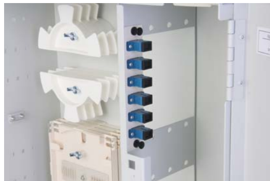
Figure 1: An unloaded LANLINXS panel demonstrates its scalability — patch plates can be added in pre-drilled holes, while splice trays and storage spool stack on posts built into the panel/chassis.
