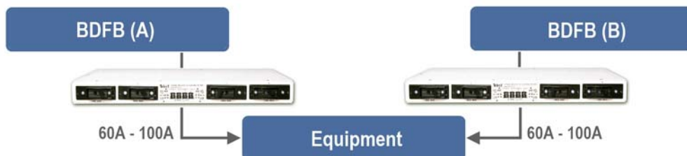
Figure 5: Typical high-current demarcation power panel application.
