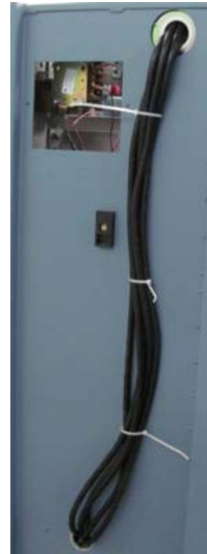
Figure 46 - Threading the Power Cables
