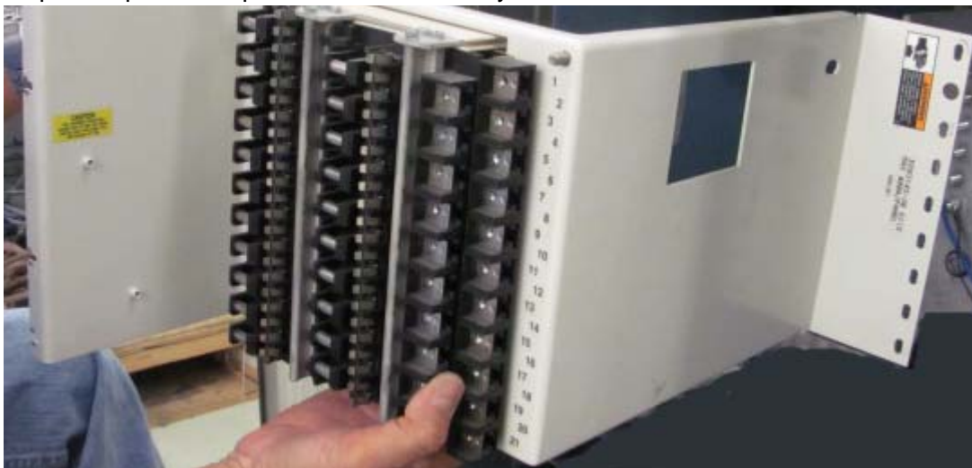
Figure 36 - Replacing the Distribution Panel
